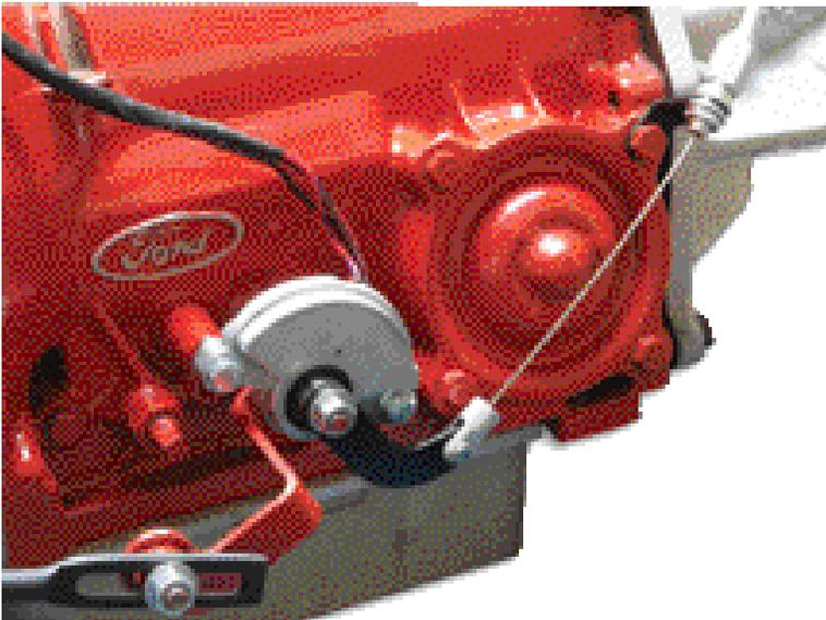
This photo shows a stock 73-77 Bronco C4 transmission with the C4 kick down cable installed. Also you can see the neutral safety switch and shift rod that goes up to the column.
